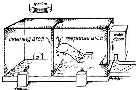
Fig. 1. The two-chambered testing cage. The mouse performs the tone detection task by crossing the barrier that separates the listening and response areas when tones are presented from the overhead speaker. The subject's movements are monitored with photocells and rewarded by activating the water dipper.
